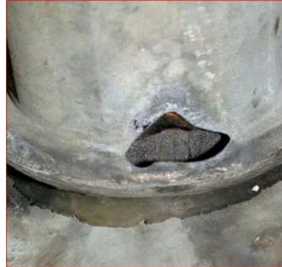
Puncture - the polymer material is ruptured due to disruptive discharge occurring through the dielectric
