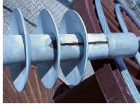
Power Arc damage – caused by high current or flashover
