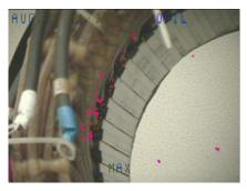
There are indicators of faults that are clear and perceived while others, not less important, are concealed or hidden. Corona, for example, is a phenomenon that indicates the existence of an electrical issue, but corona cannot be seen with bare eyes. Corona behaves as an indicator though at the same time acts as a hazardous discharge and therefore should be detected. Corona creates corrosive material such as ozone and nitric acid which erode insulation
