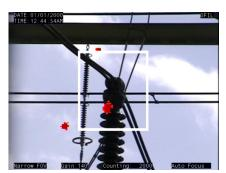
free and therefore if corona appears, it signals that the condition of that installation needs attention or else deterioration is imminent.
